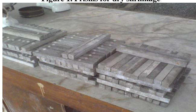
Figure 1. Prisms for dry shrinkage
